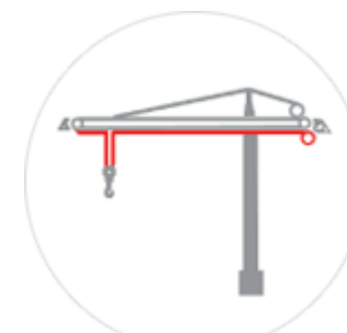
TOWER Main Hoist
