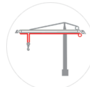
TOWER Main Hoist
